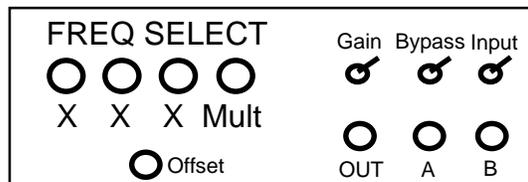
Input signals should be connected to **A**, and output signals are received at **OUT**.
