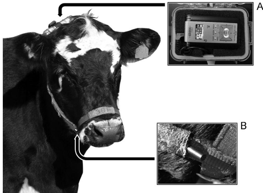
**Fig. 1.** Photograph of a heifer wearing a halter with attached digital recorder and microphone. Insets show details of: (a) recorder in the protective plastic case and (b) microphone.
